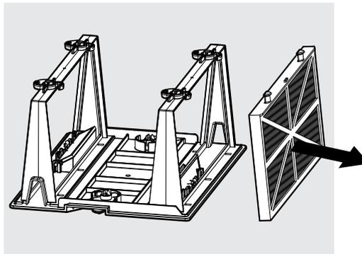
Open the clips and remove the filter.
