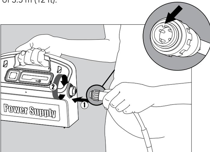
Attach the floating cable to the power supply by inserting it with the notch on the connector (1) lined up with the groove in the socket on the power supply and turning clockwise (2).
