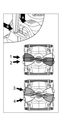
Change diagonal handle position for water line sideway movement. To adjust the handle angle:
