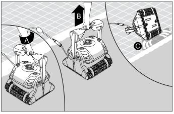
Using the floating cable, bring the Pool Cleaner to the pool's edge.
